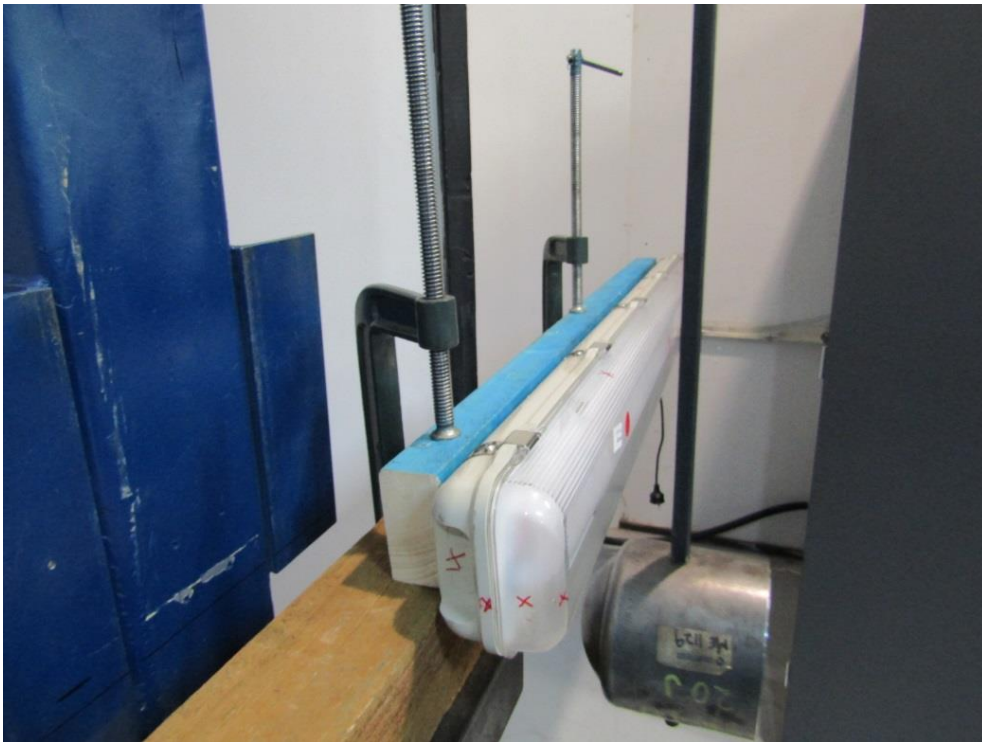
Photograph 2: Typical test setup – long face (lens)
