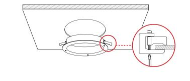
Connect luminaire to 240V plug socket and insert driver and cable into the ceiling.
