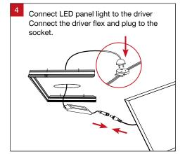
Slide the LED panel light with the driver into the surface mounted frame. Re-screw the removed side panel back to secure the panel.
