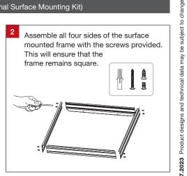
Install the surface mounted frame to the ceiling (A) with all four sides attached.
