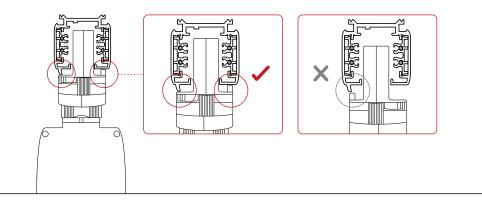
Insert luminaire into the track and move locking lever to the locked position.
