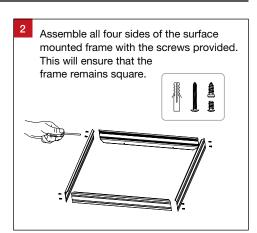
Install the surface mounted frame to the ceiling (A) with all four sides attached.
